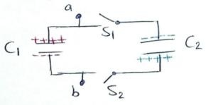
After the Switches are closed, the potential differences across the capacitors are the same and they are connected in parallel.
