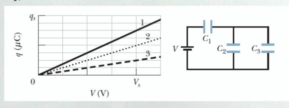
. Find each capacitance from the slope of 9 versus V curve  $C_1 = \frac{12MC}{2.0V} = 6.0MF$ ,  $C_2 = \frac{8MC}{2.0} = 4MF$ ,  $C_3 = \frac{4MC}{2.0} = 2MF$
